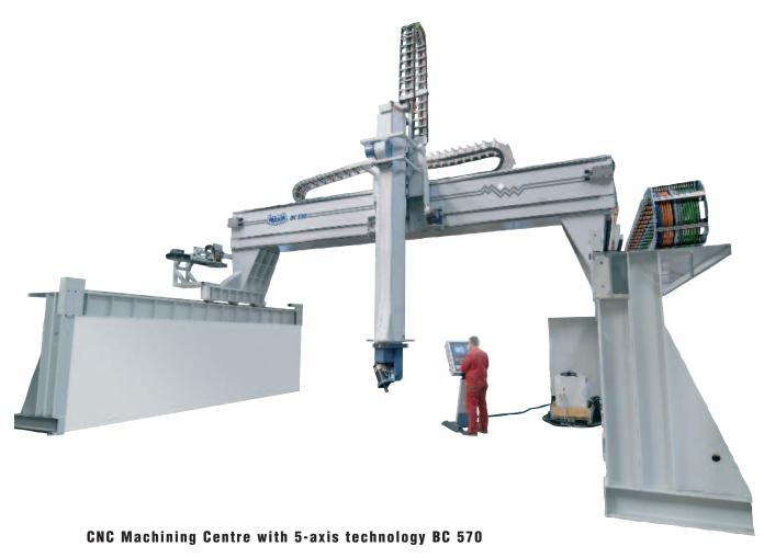
stationary centre in bridge-type design for large-pattern making
